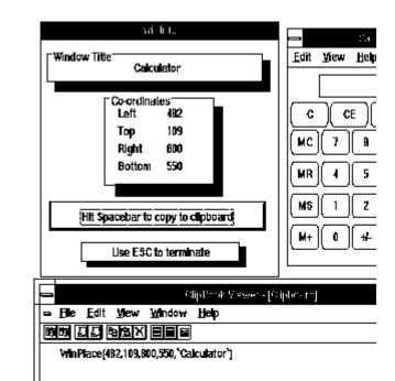
WinInfo captures relative screen coordinates. You'll need a mouse to use **WinInfo**. While **WinInfo** is the active window, place the mouse over the window you wish to create the **WinPlace** statement for, and press the spacebar. The new statement will be placed into the Clipboard. Then press the **Esc** key to close **WinInfo**.
